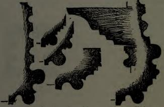
FIG. 51. Sections of marble moulding, from St. Mark's, Venice.
