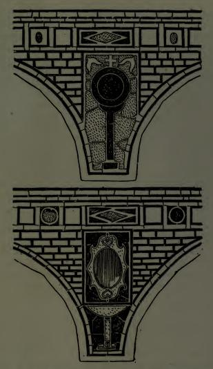
FIG. 8. Marble plating from spandrils of arches in Sta. Sabina, Rome, from a drawing by Mr. A. Christie.
