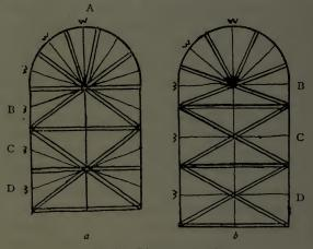
FIG. 65. Diagrams of vaults.
