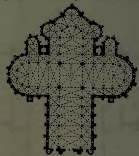
FIG. 62. Plan of destroyed church of Valenciennes with apsed transepts.
